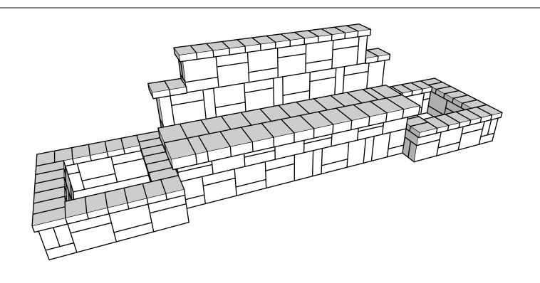
When constructing your project, be sure to keep all blocks level, square, and plumb. Use a four foot evel and check often. Starting on a level blocks together
