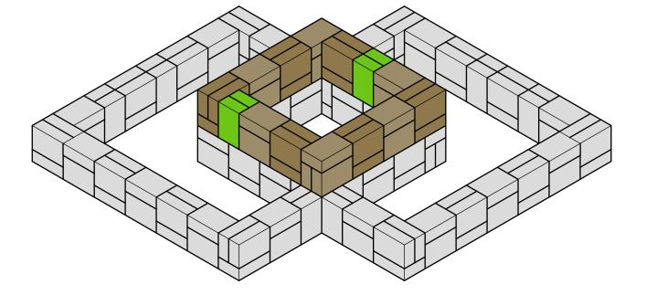
When constructing your project, be sure to keep all blocks level, square, and plumb. Use a four foot level and check often. Starting on a level foundation is key. When gluing blocks together, be sure not to use too much adhesive - this will cause the blocks to "swim." A small bead is ideal.
