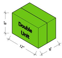
Sometimes SFUs are broken up or can't be used. The Double Unit is the next preferred unit. Double Units are grouped for strength and speed in construction. They are always represented in green.
