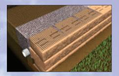
When the weight of the units alone is insufficient to resist soil loads, horizontal layers of VERSA-GRID or other types of geogrid are used to reinforce soil behind walls. VERSA-LOK retaining walls can be built to heights of 50 feet or more with proper soil reinforcement and design assistance from a licensed professional engineer.
